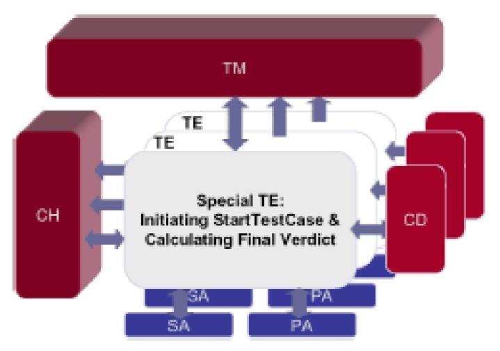
The distributed test system architecture defined in TCI standard
