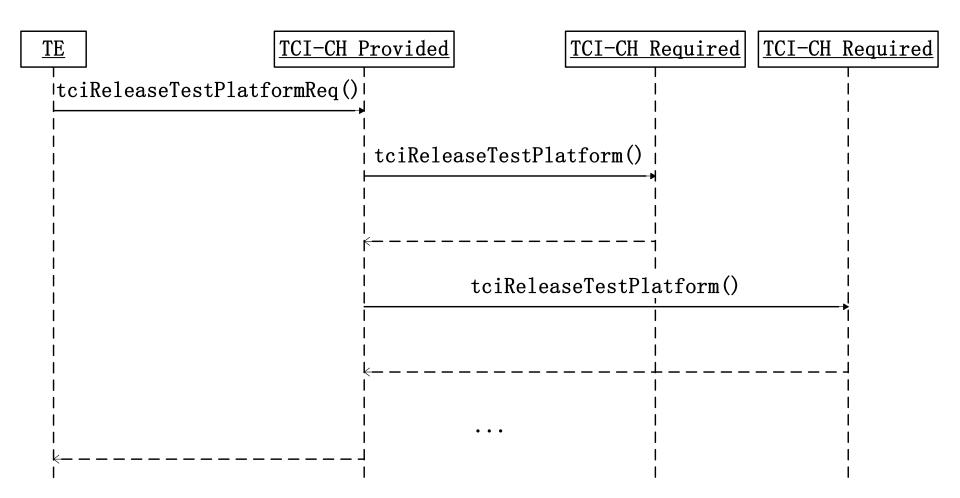
Use scenario - release test nodes after finishing test suite execution
